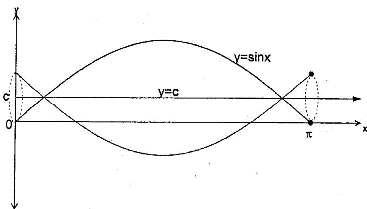
The arch  $y = \sin x$ ,  $0 \leq x \leq \pi$ , is revolved around the line  $y = c$  to generate the solid shown.
